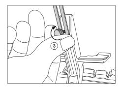
Insert the fixing knob (3) and tighten it just enough so that it stays in place but the display holder can be moved.
