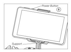
Place the display on the support with its buttons facing upwards. Adjust the height of the display holder tighten the fixing knob.
