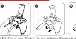
Pull off the top edge of the fixed clip, then pull down until the edge is removed from the gamepad. Move the fixed clip down and push it back at the same time 3. Move the whole of fixed clip back, then the detachment is finished
