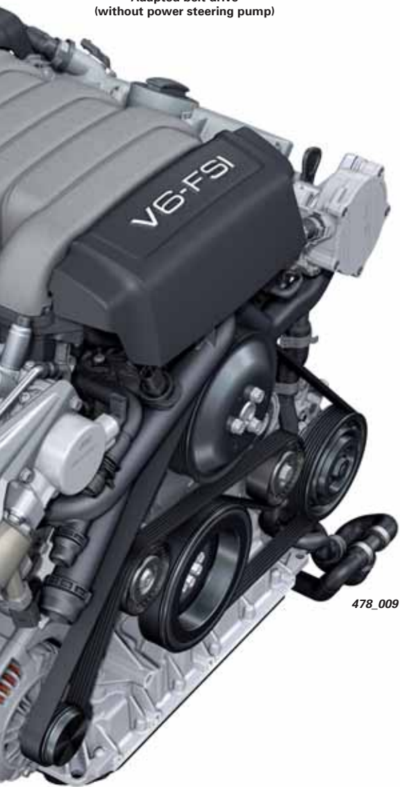
Adapted belt drive (without power steering pump)
