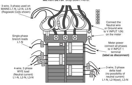
NOTE: The VerifEye meter series uses the NEUTRAL terminal as a voltage reference. For systems without a neutral conductor, Leviton suggests connecting a ground wire to this terminal. If the neutral terminal is left open, L-L measurements will be accurate, but L-N measurements may not be symmetric. If a ground wire is connected to the NEUTRAL terminal, <2mA will flow into the ground wire.
