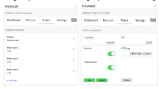
4. No need to manually type in the RFID tag number – you can scan it with the device, and automatically assign it to the selected user in Heimdall app settings.
