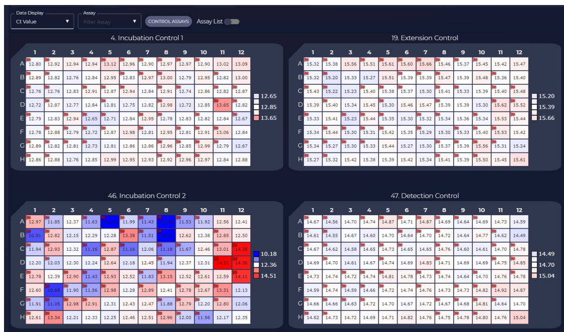
Figure 15. Ct values that show primer contamination of Incubation Control 2.
