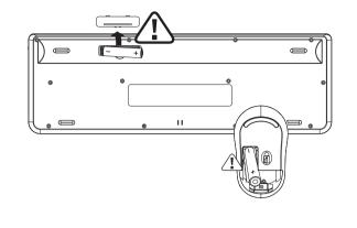
① Open the battery cover, remove the insulation rubber, install the battery (note the +/- electrodes) 打开电池盖, 撕掉绝缘胶皮, 装入电池(正负极正确)
