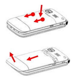
Remove the battery from the phone by lifting from the bottom and pulling out.
