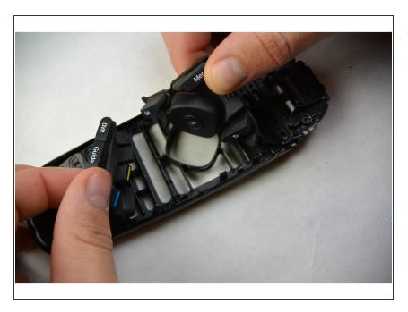
From the front of the remote, remove the buttons. Clean or replace the necessary buttons.
