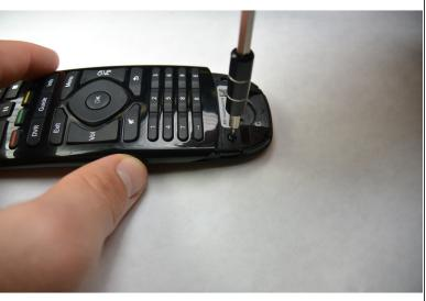
With the PH00 bit, remove both of the 4mm Phillip screws on the remote.
