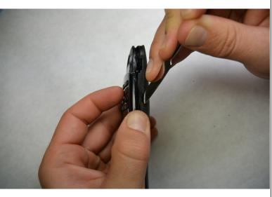
Using a metal spudger, pry the remote. Maneuver around to separate both sides.
