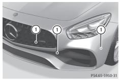
Sensors on the front bumper, left-hand side (example)
