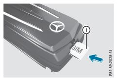
► With the contact surface facing down, insert SIM card ① into the SIM card slot until it engages.
