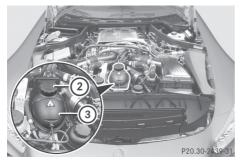
Example: checking the coolant level
