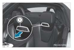
The blower setting of AIRSCARF vent (1) can be adjusted using the AIRSCARF button (⊳ page 89).
