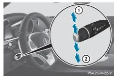
➤ To adjust the set speed in 10 km/h increments: briefly press the cruise control lever up ① beyond the pressure point for a higher speed, or down ② for a lower speed.
