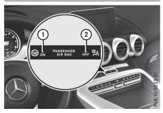
PASSENGER AIR BAG ON indicator lamp ① and PASSENGER AIR BAG OFF indicator lamp ② are part of the automatic deactivation system of the front-passenger front airbag.
