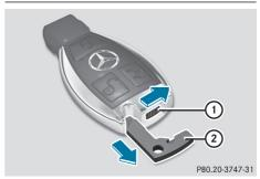
▶ Push release catch ① in the direction of the arrow and, at the same time, remove emergency key element ② from the key.
