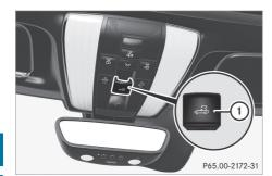
▶ To open: push soft-top switch (1) upwards until the soft top is fully opened. In the multifunction display, the Top in operation message appears.
