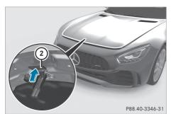
▶ Reach into the gap, pull bonnet catch handle 2 up and lift the bonnet. If you lift the bonnet by approximately 40 cm, the bonnet is opened and held open automatically by the gas-filled struts.
