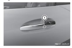
▶ Touch recessed sensor surface (1) on the door handle until the side windows are fully closed.
