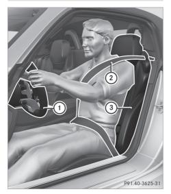
Ensure the following when adjusting steering wheel (1), seat belt (2) and driver's seat (3):
