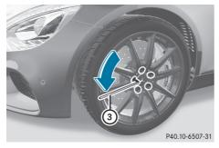
▶ Using wheel wrench ③, loosen the bolts on the wheel you wish to change by about one full turn. Do not unscrew the bolts completely.
