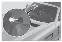
Lane Keeping Assist monitors the area in front of your vehicle by means of multifunction camera (1) attached at the top of the windscreen. Lane Keeping Assist detects lane markings on the road and can warn you before you leave your lane unintentionally.
