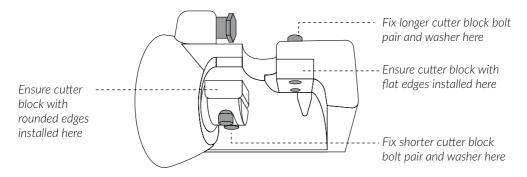
Check cutter block bolts for tightness before each use. Use protective gloves when handling cutter blocks as edges are very sharp.
