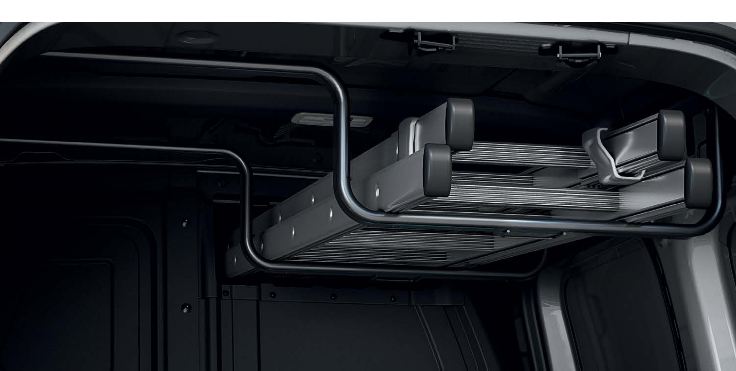
easy inside rack* with a load length of 2088mm and 2514mm
