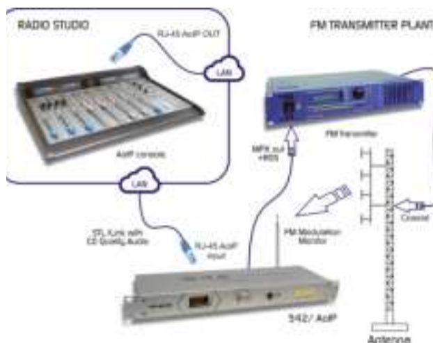
Figure 39: Basic diagram for streaming connection
