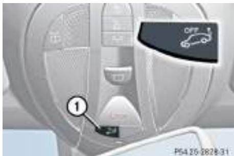
① Tow-away alarm off button
