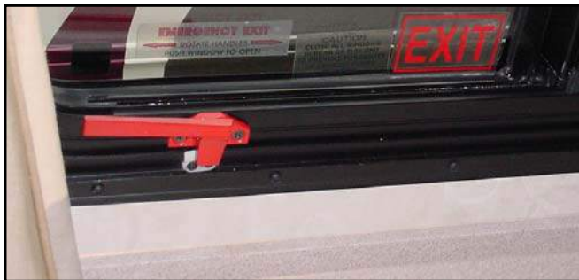
Figure 13-2. Bedroom Emergency Exit Window
