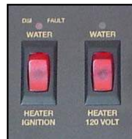
Figure 4-16. Water Heater Switches
