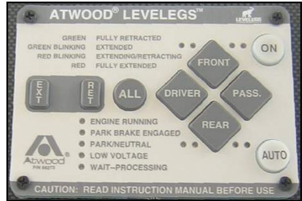
Figure 9-6. Leveling Control Panel on Dashboard
