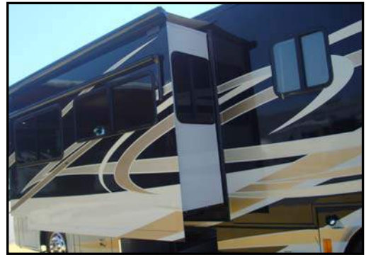
Figure 8-2. Typical Slide-Out Fully Extended
