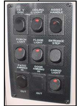
Figure 9-8. Entrance Step Switch (right middle)
