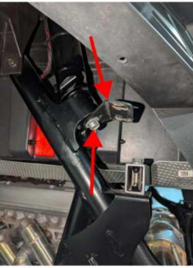
If running a license plate, right now is a good time to install it to the bumper while access to the backside of the hardware is much easier for the installer, next remove the outer two bolts located below the muffler and set aside for now. next remove the two bolts that secure rear section of the cage to the frame and install the supplied plates as shown with the break towards the ground, leave these bolts slightly loose for now to ease getting the other hardware started.
