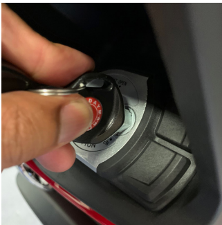
Take the back of the key. And put it in the ignition lock
