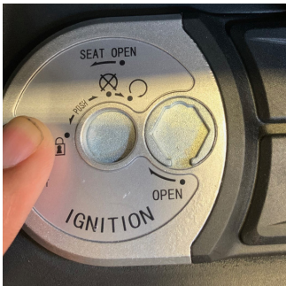
Push the ignition lock button to close ignition
