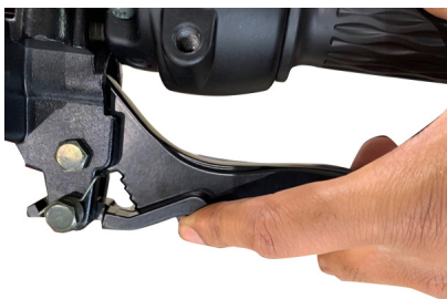
While holding brake pull brake lock lever into the grooves.
