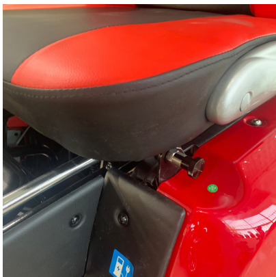
While Holding the seat latch out slide the chair back
