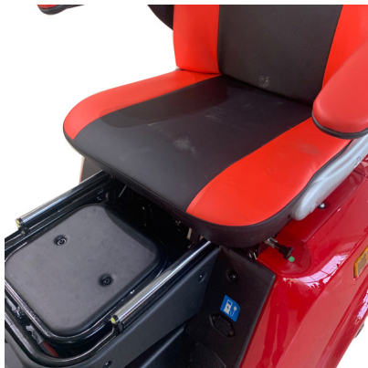
While Holding the seat latch out slide the chair back
