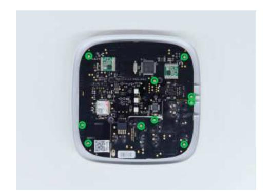
**6.** Carefully remove both boards, keeping them in the same plane and not disconnecting them. There is a connector between boards: do not break it.
