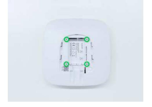
**5.** Remove the screws attaching the boards to the device body.
