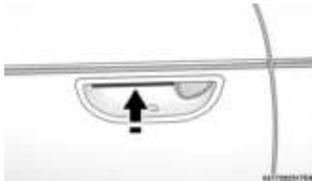
Lift The Door Handle To Unlock
