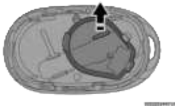
Removing Battery Cover
