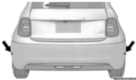
Radar Sensors Location
