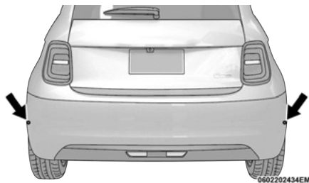
Radar Sensors Location
