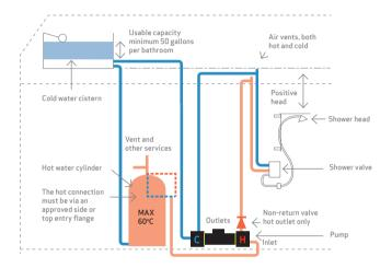
Right Pump twin ended positive head with up and over pipework and natural flow of 1Litre/min per side.
