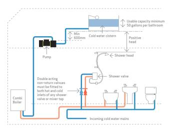
Tank-fed, pressurised cylinder or combi boiler system with Right Pump single ended universal pump to boost the hot supply water pressure and cold water mains supplies 'cold' to shower, bath, basin and toilet.
