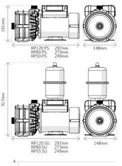
All Right Pumps have the standard inlet/outlet configuration for ease of replacement.
