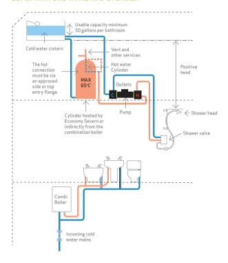
Combi boiler system with Right Pump twin ended positive head to boost the shower from a cold water supply tank and a direct cylinder.
