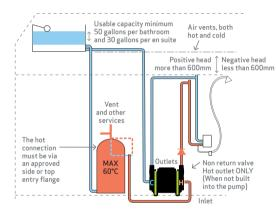
Negative head When the distance between the cold water storage cistern and the shower head is 600 mm or less, or when the natural flow is poor or less than 2 litres ner minute of combined hot and cold it is possible a negative head pump may be required.
