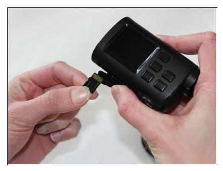
When putting a micro SD card back into the device, be sure to place the exposed metal side up, as well as have the device LCD screen side up.
