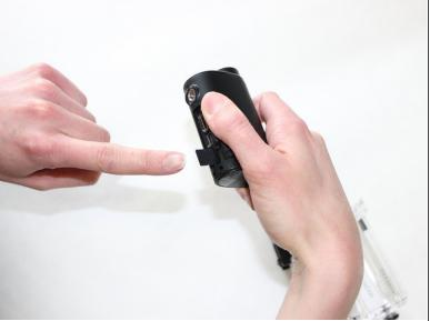
• To remove the micro SD card from the device, gently push the SD card and release. The SD card will pop out.
