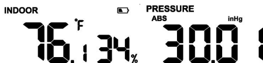
Figure 27: Indoor temperature, humidity and pressure
