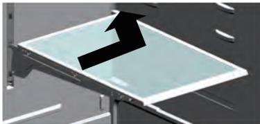
2. To reinstall a shelf, gently slide the shelf back into the refrigerator compartment, and then lower the shelf onto the shelf guides so that the hooks fit behind the rear guides.
