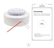
6. Press RESET for 5 seconds with PIN when configuration network, indicator flashes slowly, start manual network configuration mode. Input WiFi account and code to add device.
