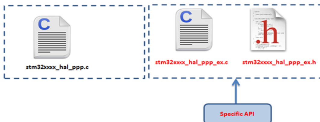
Figure 2. Adding device-specific functions
