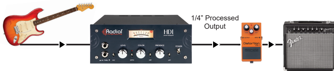
Connecting an instrument and an amplifier to the HDI
