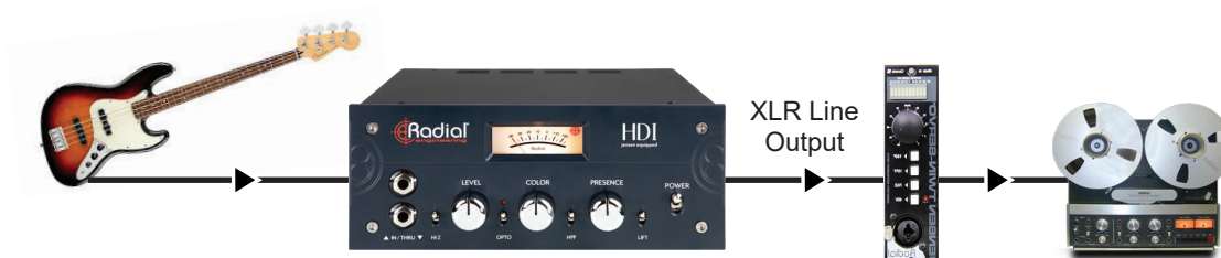
Using the HDI to overdrive a microphone preamp
