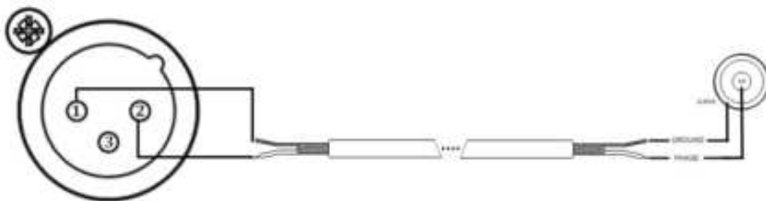
2. Connection from balanced output to unbalanced input
