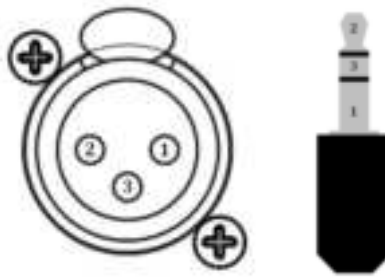
4. Numbering pins connector XLR and Jack ST
