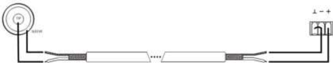
4. Connection of unbalanced output to balanced input
