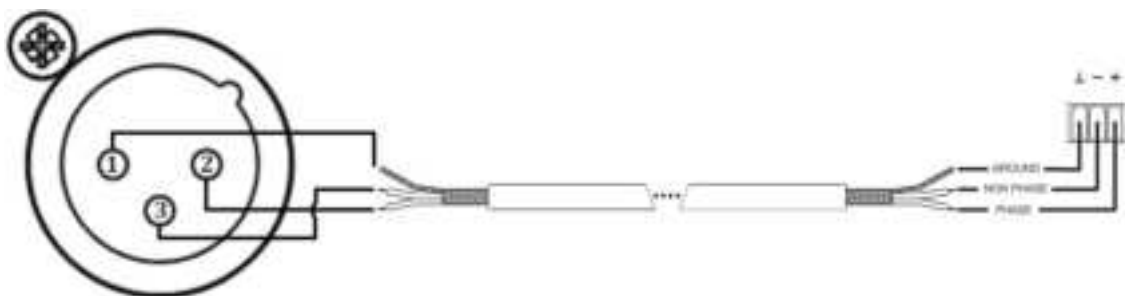
1. Connection from balanced output to balanced input
