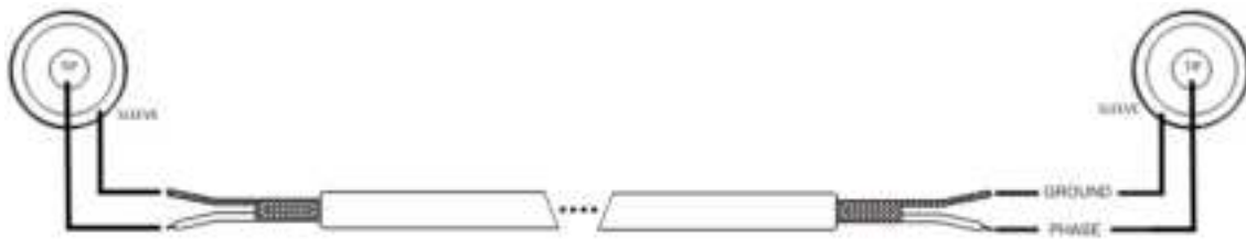
3. Connection from unbalanced output to unbalanced input
