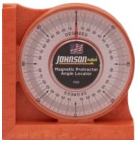
Measuring angles is a snap with Johnson's magnetic angle locator. It features a high-impact molded body and an extrastrong ceramic magnet that sticks to ferrous metal surfaces, while the v-groove edges fit perfectly onto pipe and conduit. Easy to read increments show 0-90° in all four quadrants on the durable acrylic lens, and the sides are marked with length graduations for convenience - one leg shows inch graduations while the other leg shows metric graduations.
