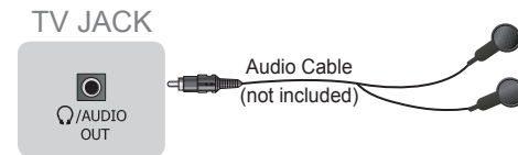
Figure 10. Diagram that shows how to connect headphones to the TV
