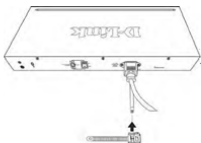
Figure 3-3. Slide the Retainer through the Tie Wrap
