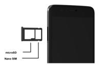
2. Gently pull out the SIM card tray gently. Place the Nano SIM card in card slot 1. If you have a microSD card (sold separately) place it in card slot 2.
