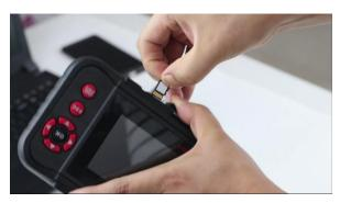
4. Put the TF card into the card reader and connect it to the computer.
