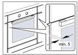
2.Screw the device in place.
