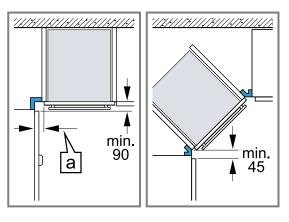
To ensure that the appliance door can be opened, you must adhere to the minimum dimensions for corner installation. The size depends on the thickness of the furniture front and the handle.
