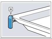
Remark:When fully extended, the telescopic rails click in. Slide the telescopic rails back into the interior with a light push.
