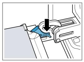
aThe locking levers are closed. The devicedoor is secured and cannot be removed. 5.Close the door of the device.
