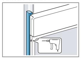
4. Secure the device with adequate screws.
