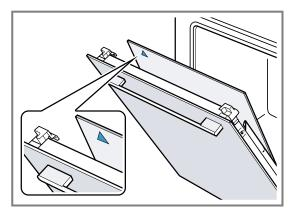
1.Slide the first intermediate pane into the lower holder and ① position it at the top.
