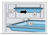
3.To install the e for sliding heights with telescopic accessory scope rails ails, pull out the telescopic rails.
