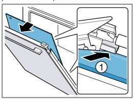
Note:The intermediate pane positions itself automatically by means of the rotating movement and spacer.
