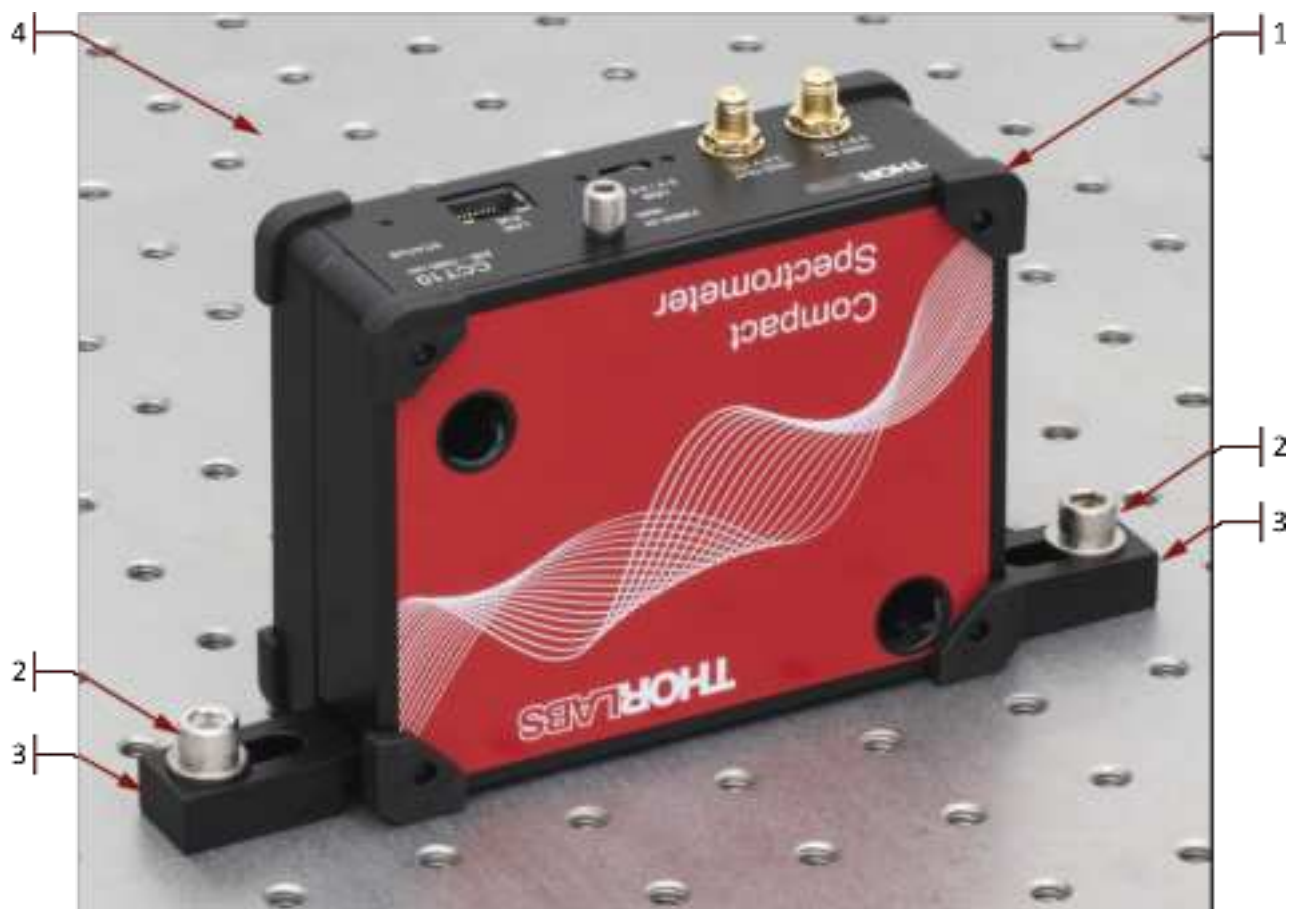
Figure 4 Mounted CCT Spectrometer with Compact Table Clamps on Breadboard
