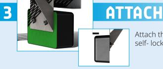
Attach the CLT20-Ex using self-locking nuts.
