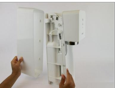
Pull the outer cover away from the front of the device.
