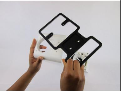
Remove the four 17.8 mm screw from the bottom metal base using a Phillips #1 screwdriver.
