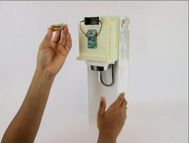
Remove the old battery and replace it with a new 3V lithium battery.
