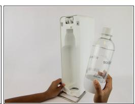
Remove the soda bottle and the CO2 canister from the machine.
