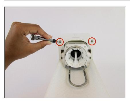
Remove the two 18.2 mm screws from the bottom of the front cover using a <u>Phillips #1 screwdriver</u>.
