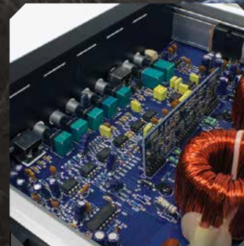
Accu-Cross™ crossovers and adjustments for sound shaping
