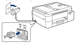
Insert the telephone line cord into the socket marked LINE.
