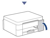
After installing all of the four ink cartridges, close the ink cartridge cover.
