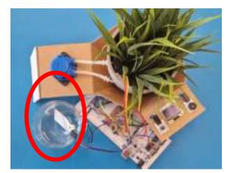
Place the suction hose in the container with water and the other hose of the paristaltic pump to the plant
