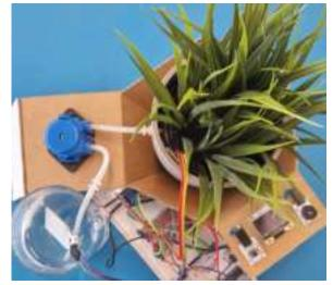
You can manually operate the peristaltic pump by pressing the tactile switch. This will only work when there is enough water in the container. The Buzzer will sound when the Water level is too low. The Oled will display if the water Level is OK or too Low. You will also get a reading from the moisture level of the plants soil. The peristaltic pump will operate automatically if the value is below 400. You can change these values by modifying the source code on the GitHub page (QR code on top).
