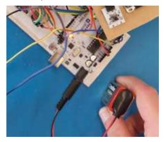
There will be different values displayed on the OLED screen. Place the Moisture sensor in the soil of a plant or flower. Place the Water level sensor in a container with water.
