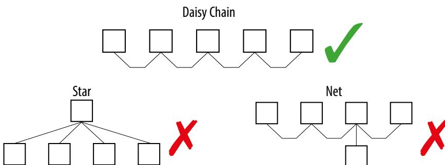
No more than two wires can be connected to each terminal, ensuring that a "Daisy Chain" (in series) or "straight line" (direct) configuration is used. Star or network (open) connection is not recommended, as reflections within the cable can cause data corruption.
