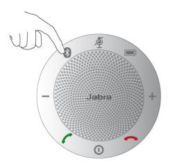
2. Insert the Link 360. The Bluetooth light flashes blue when it is in pairing mode. It can take up to one minute for your Jabra Speak 510 and Jabra Link 360 to pair. Note: You can also enable pairing mode for the Link 360 in Jabra Direct.
