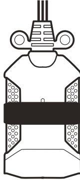
Securing the CN800 using a magic tape
