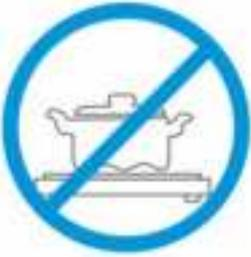
Do not place rough or uneven appliances, which may damage the ceramic surface .
