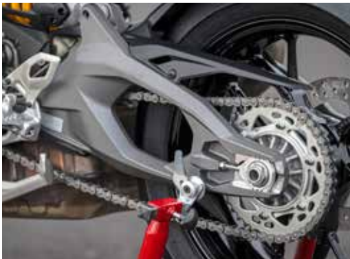
Swingarm It's out with the single-sided swingarm and in with a delicate V4 Panigale-style hollow ali double sider, for less weight and more lateral flex.
