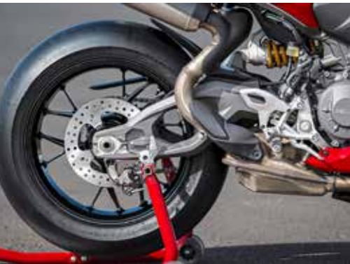
Wheels New cast ali 17in wheels with Y-shaped spokes are shod with Pirelli Diablo Rosso IV tyres. Rear has gone up from the old 180/60 to a 190/55.
