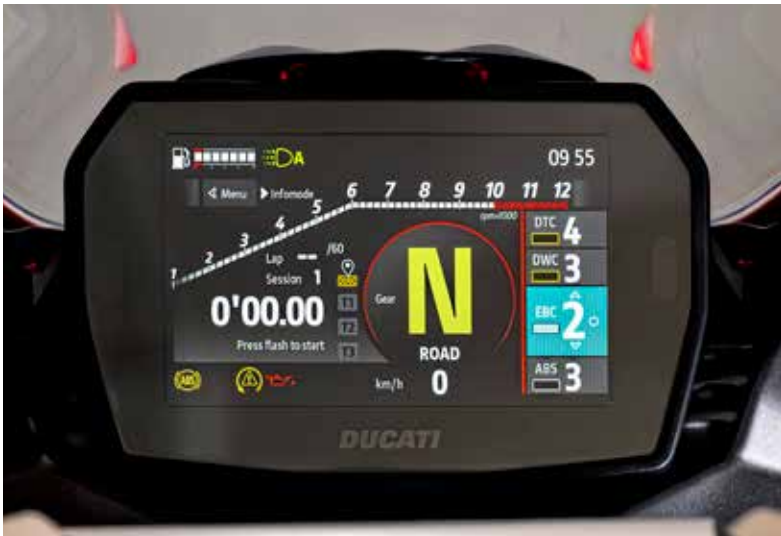
TFT New 5in colour dash has a 16:9 aspect ratio and three display modes: Road, Road Pro and Track, highlighting the relevant information you need.
