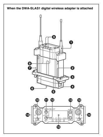
**1** Antenna and antenna connector (SMA type) Connect the supplied antenna here.
