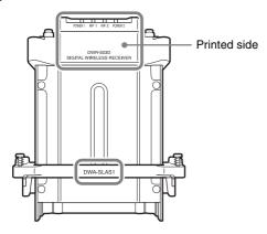
**2** Use the screws included with the DWA-SLAS1/SLAU1 to secure the bracket to the receiver.
