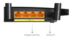
**Step2:** Press the WPS button on the router for 3-5 seconds. The router indicator light will begin to flash, letting you know it is searching for a device to connect.
