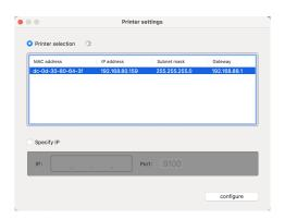
**Note:** If the network info does not show up, choose "**Specify IP**" ->Input IP address and Port (Note: find the IP address and Port info from **[WiFi configure]** label)
