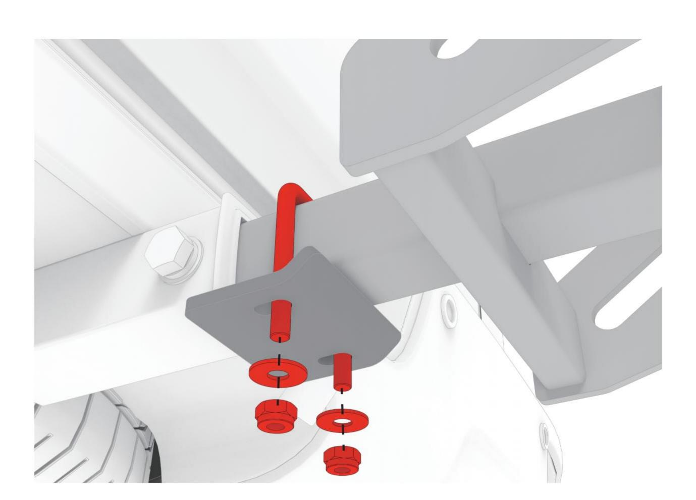
Tighten the nut on the **U-shaped shock absorption(3)** mechanism to reduce vibrations.
