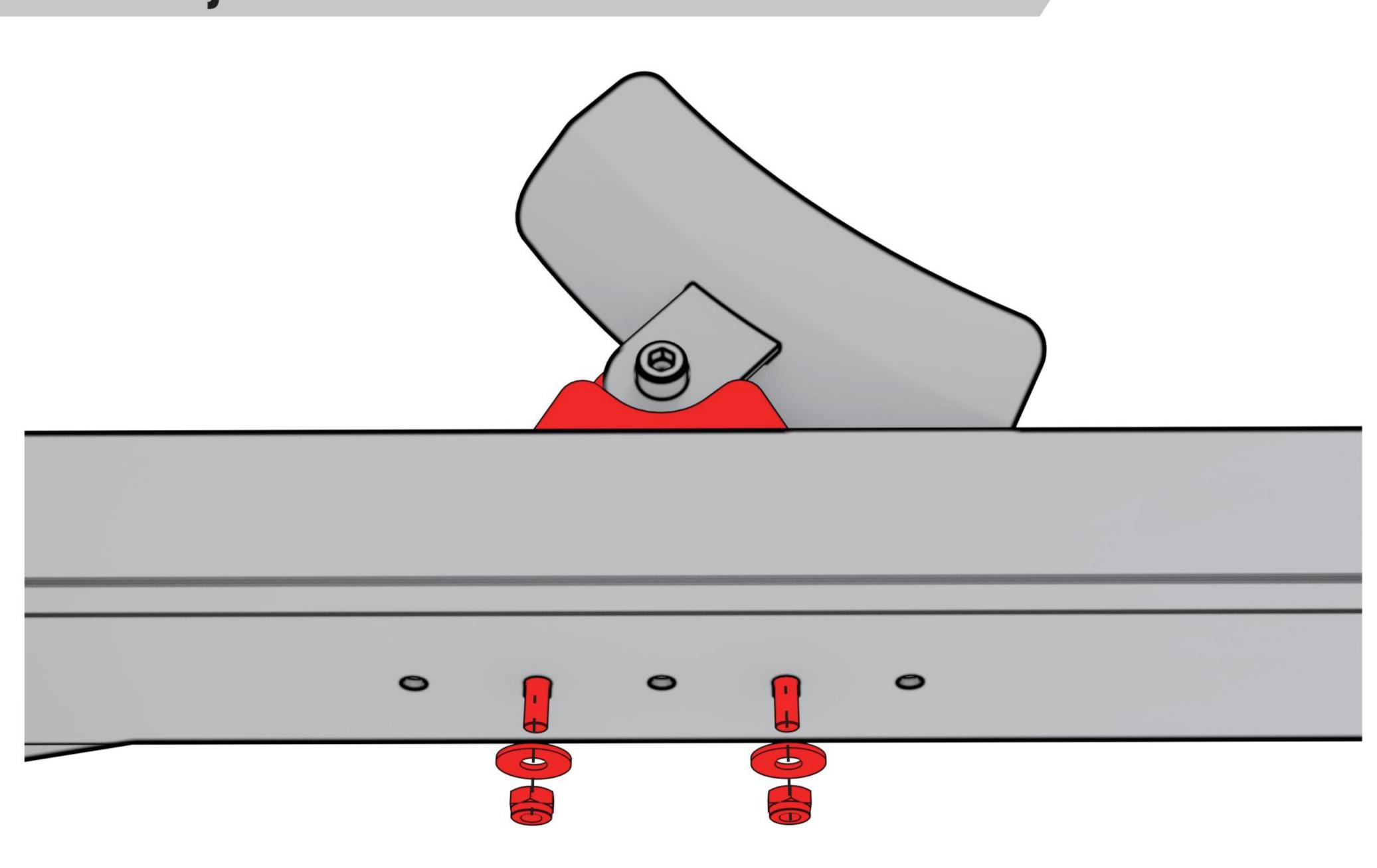
The position of the Front Wheel Holder can be adjusted according to your needs. There are three optional positions.
