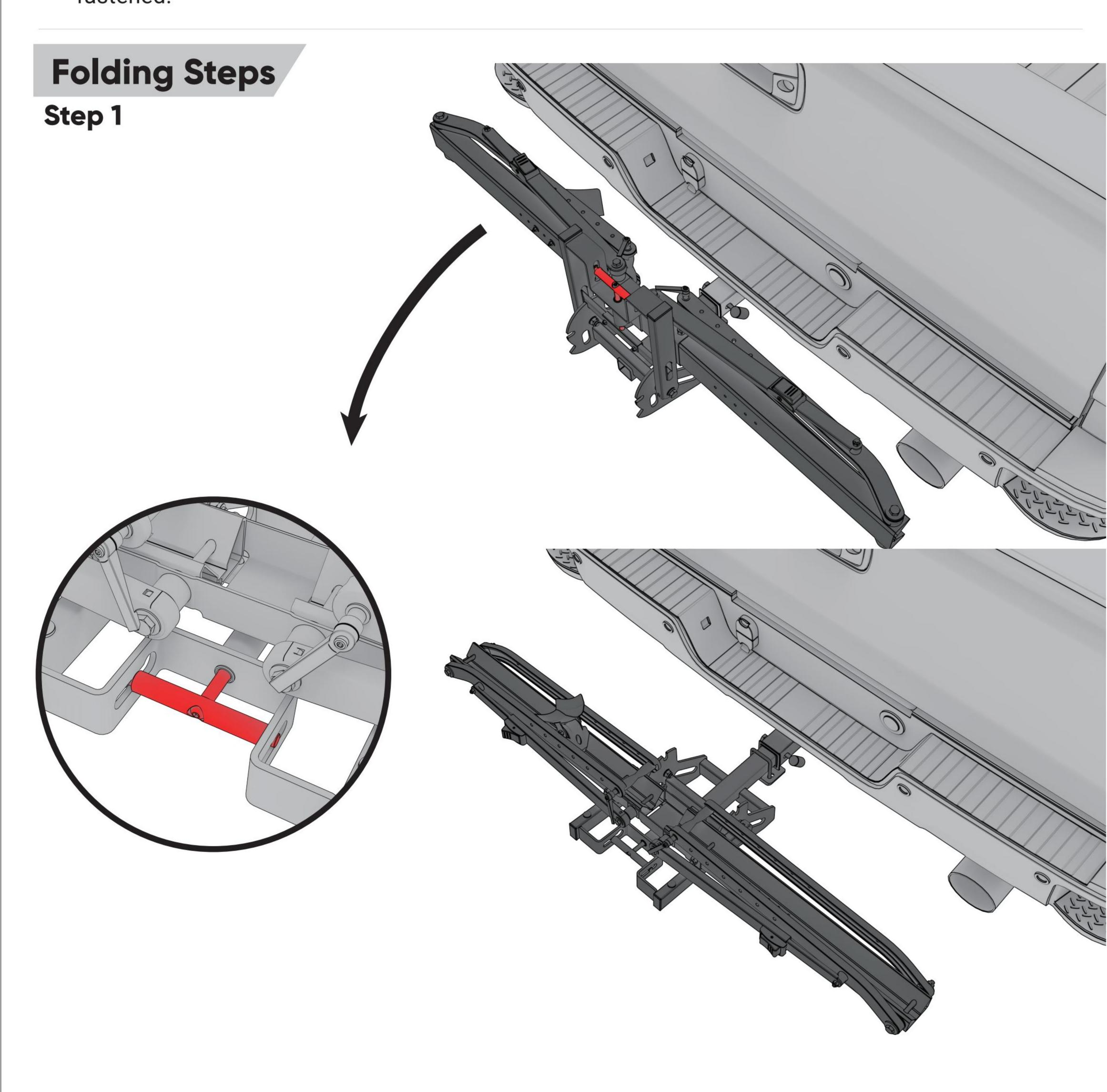
Hold the Handle Assembly and lower the bike rack to the lowest position, making sure the gear
