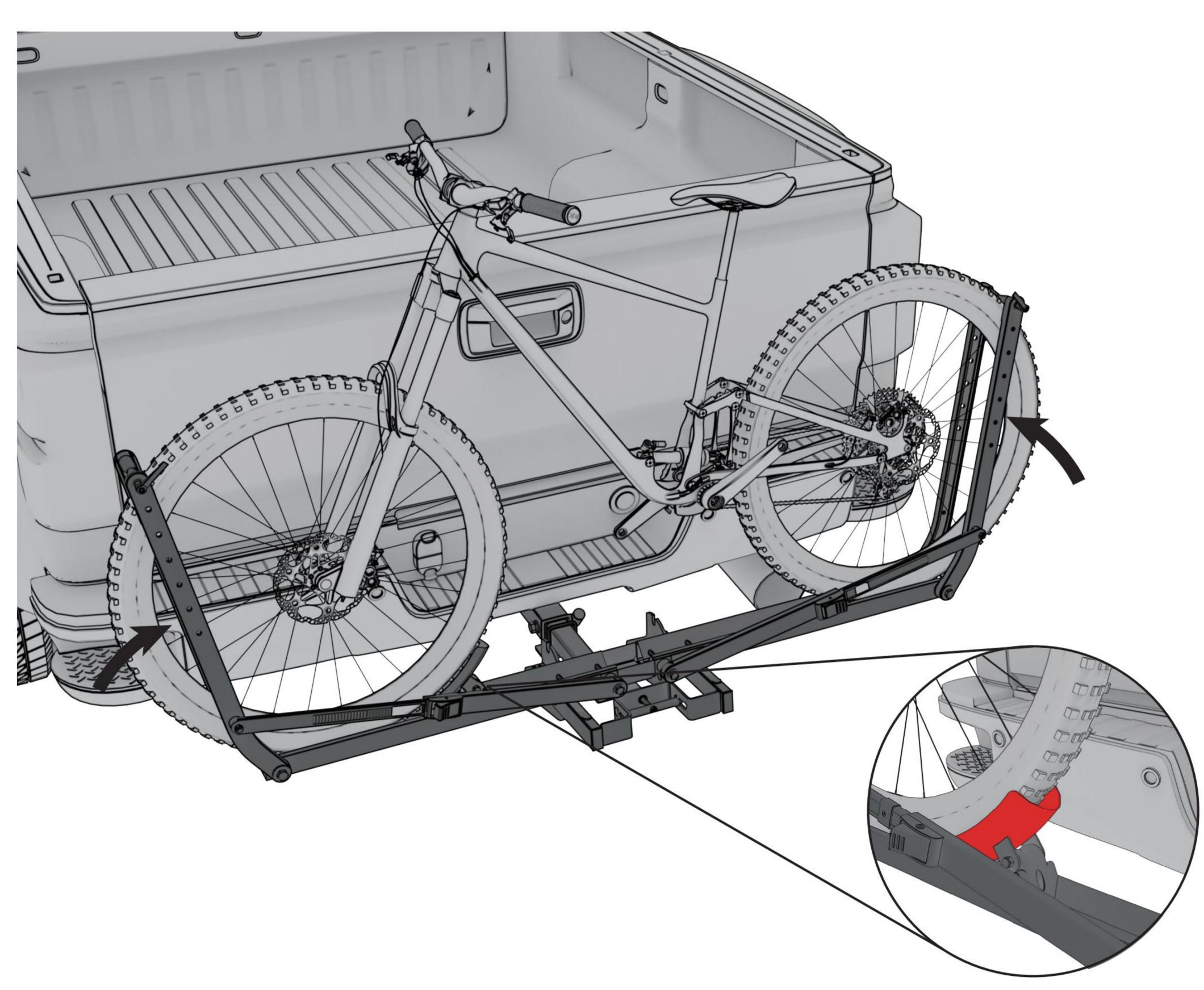
Install the bicycle on the Bike Rack, place the front wheel against the Front Wheel Holder, and tighten the Bent Arms on both sides to ensure that the front and rear wheels of the bicycle are firmly fixed.
