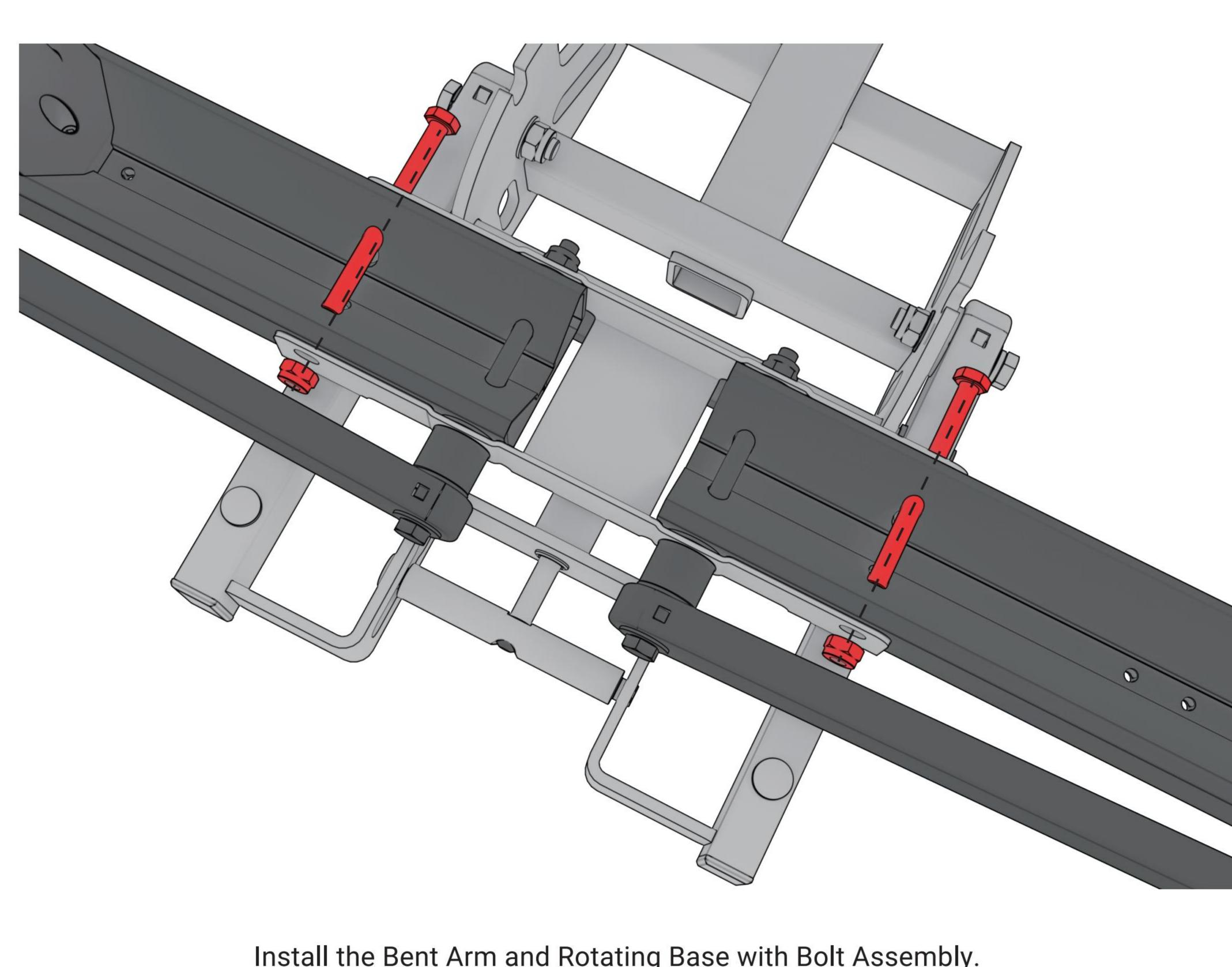
Install the Bent Arm and Rotating Base with Bolt Assembly.
