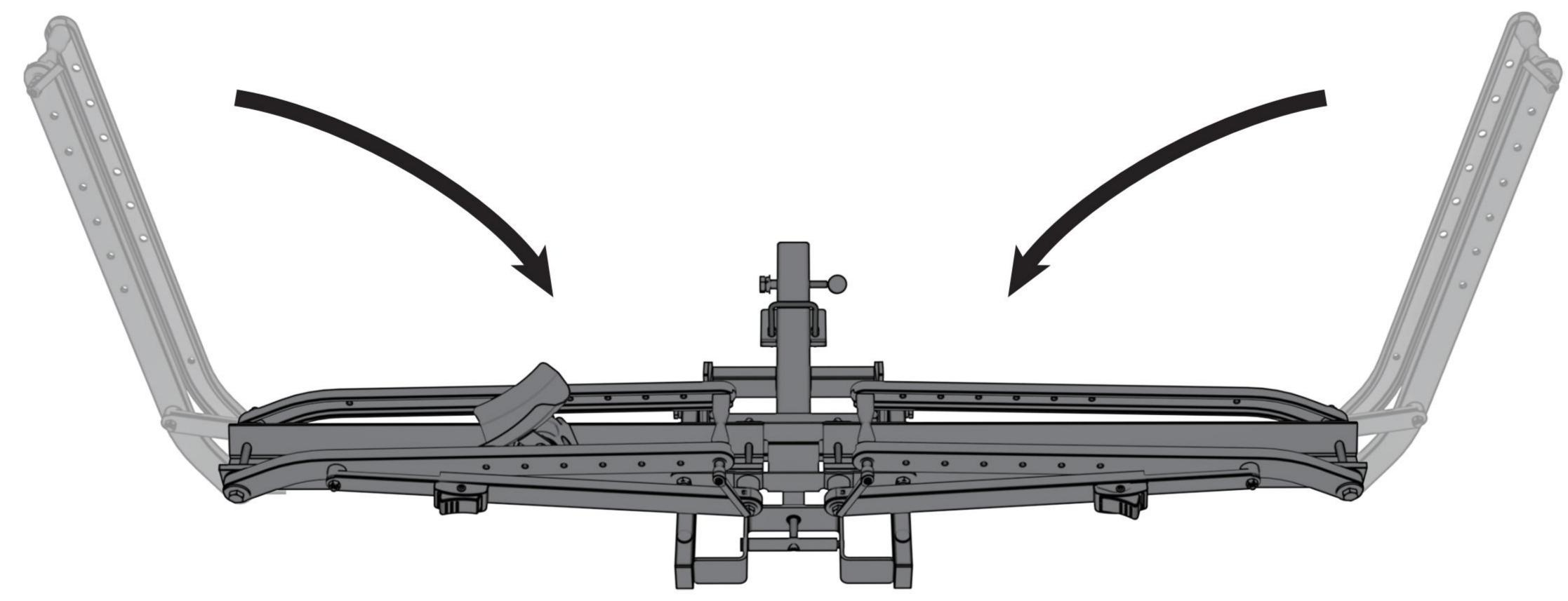
No need to press Adjustment Button when folding the bent arm assembly.
