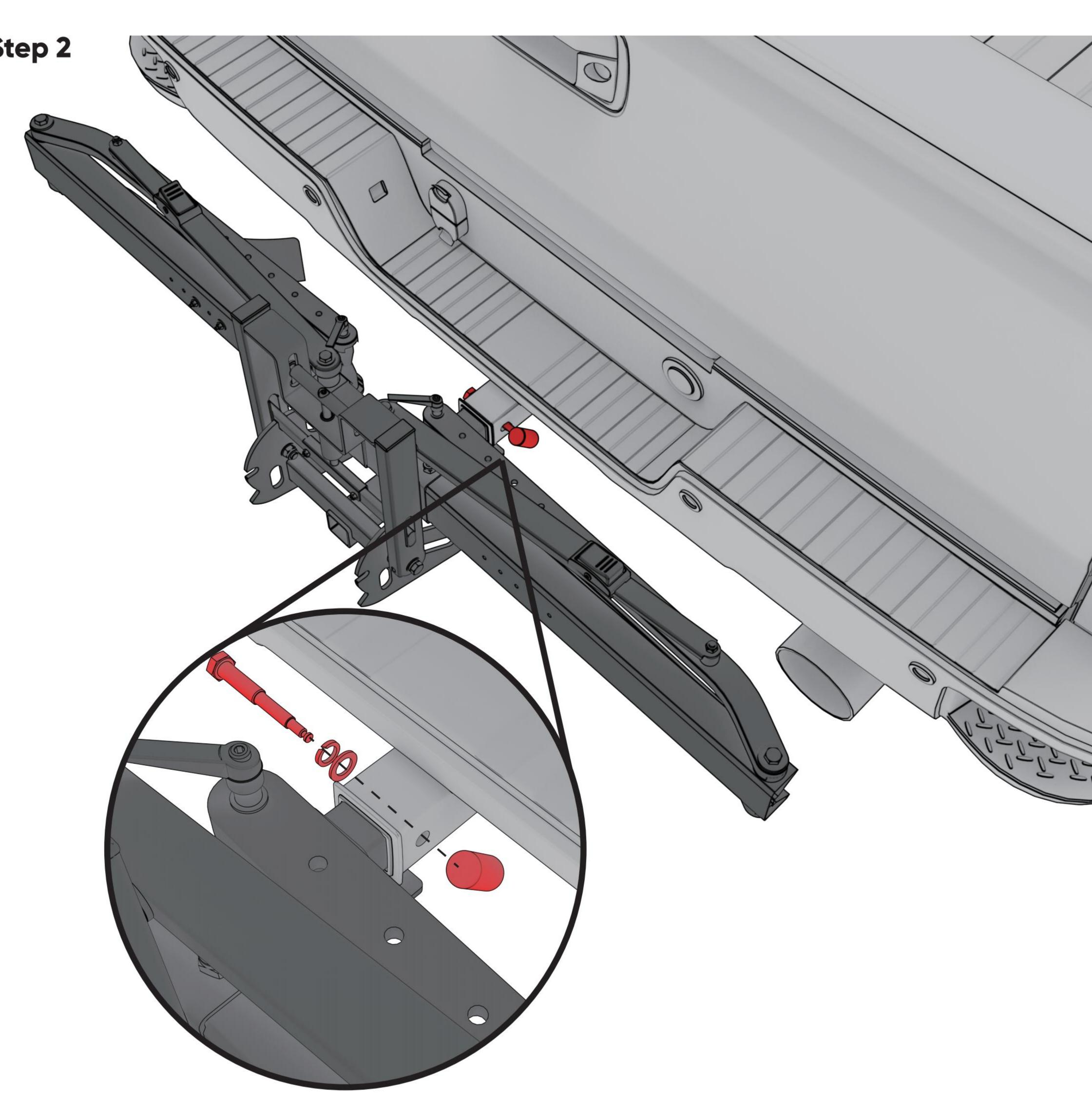
Insert the Bike Rack into the vehicle receiver and Place an Pin Lock (4), through the Spring Washer and Flat Washer and the aligned holes. Insert the lock head and ensure it is securely fastened.
