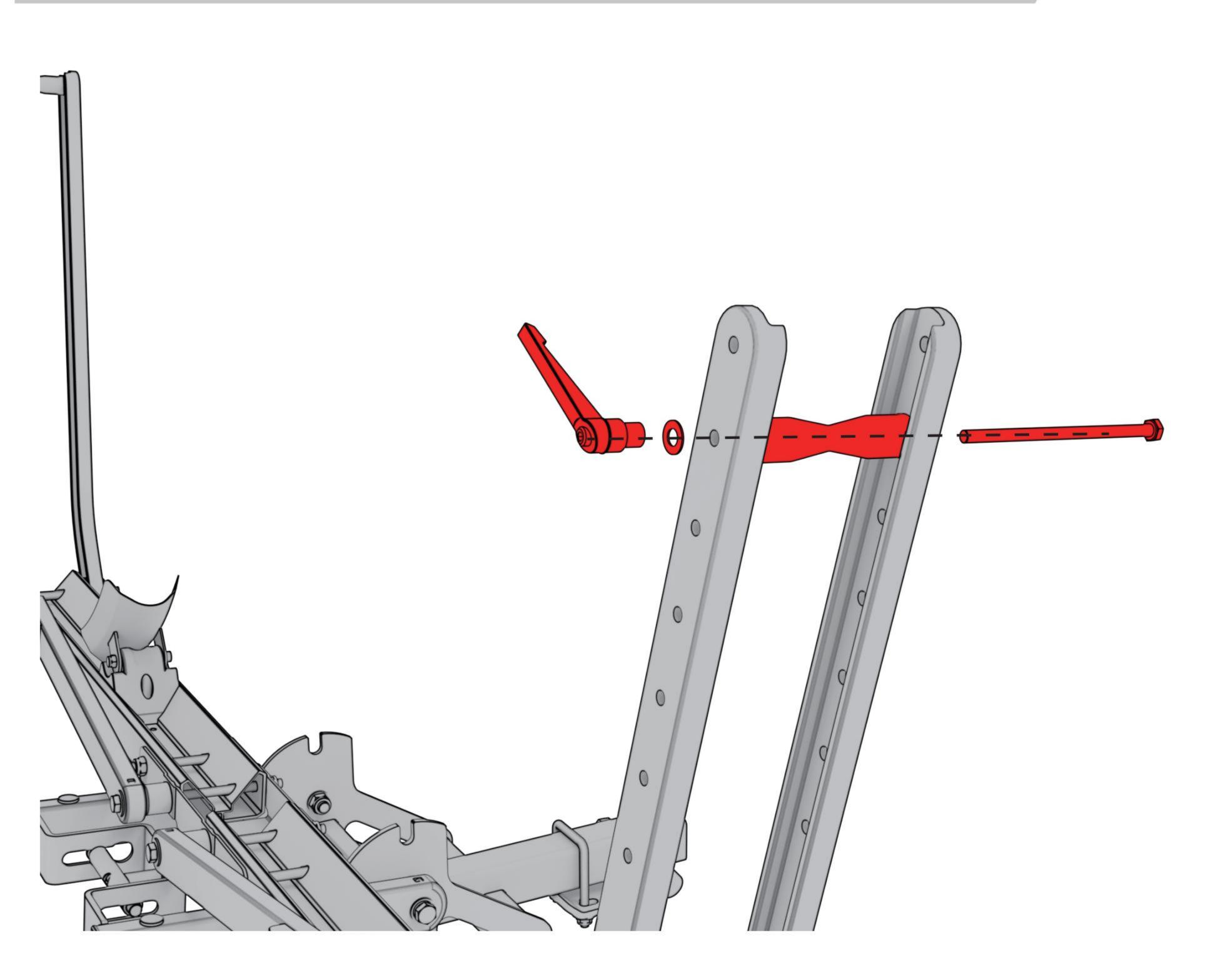
The position of the Adjustment Lever can be adjusted according to your needs. Loosen it counterclockwise and tighten it clockwise.
