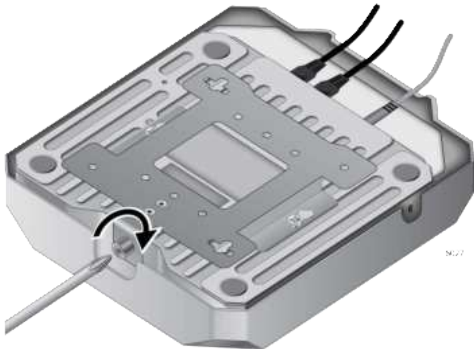
Figure 27. Tightening the Mounting Bracket Thumbscrew
