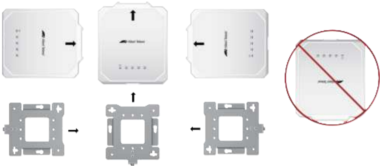
Figure 26. Seating the Access Point on the Mounting Bracket
