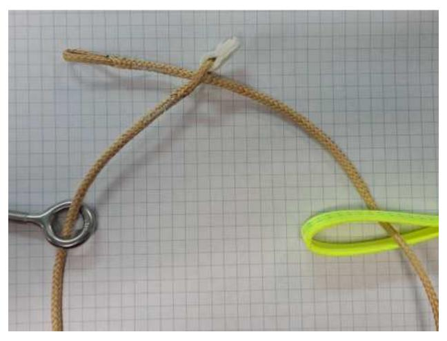
Step 1: Route the looped end through the items being linked together and back through the looped end.
