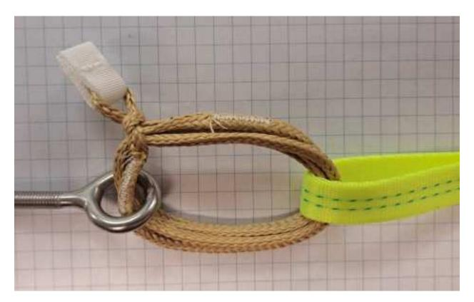
Step 5: Push the loop down past the stopper, and ensure the looped end is tight and low on the stopper end's loop. Tension the link by either pulling the link in opposite directions with your fingers or by pulling the linked items apart. NOTE: It is very important that the looped end "seats" itself tightly under the stopper.
