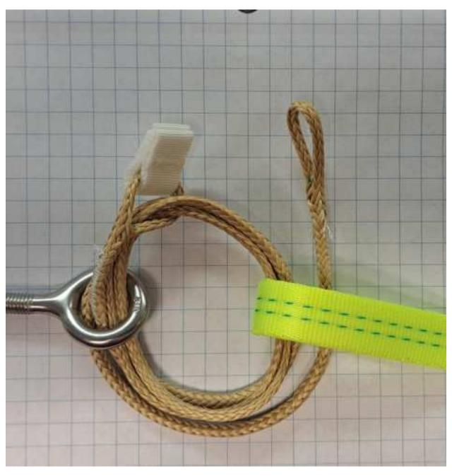
Step 3: Before securing the soft link, make sure that the looped end is routed through the items to be linked together and through the stopper end, with each pass.
